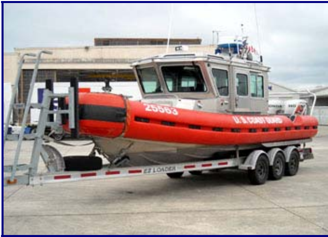
USCG DEFENDER Class boat used for SARs and other Assigned tasks by CG Sector Jacksonville
